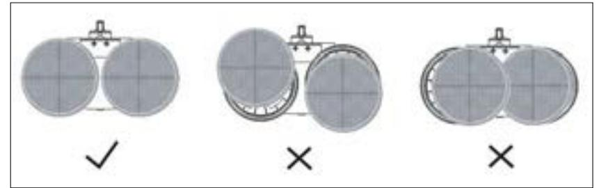
Always ensure the pads are located centrally on each rotating base.
