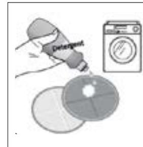
When machine washing apply a little detergent to each pad directly.
